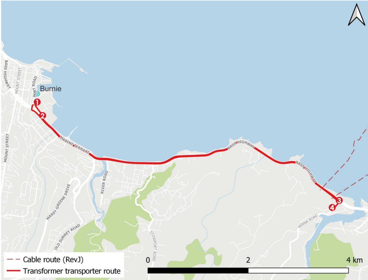
Figure 7-1: Transformer Transporter Swept Path Assessment Locations
